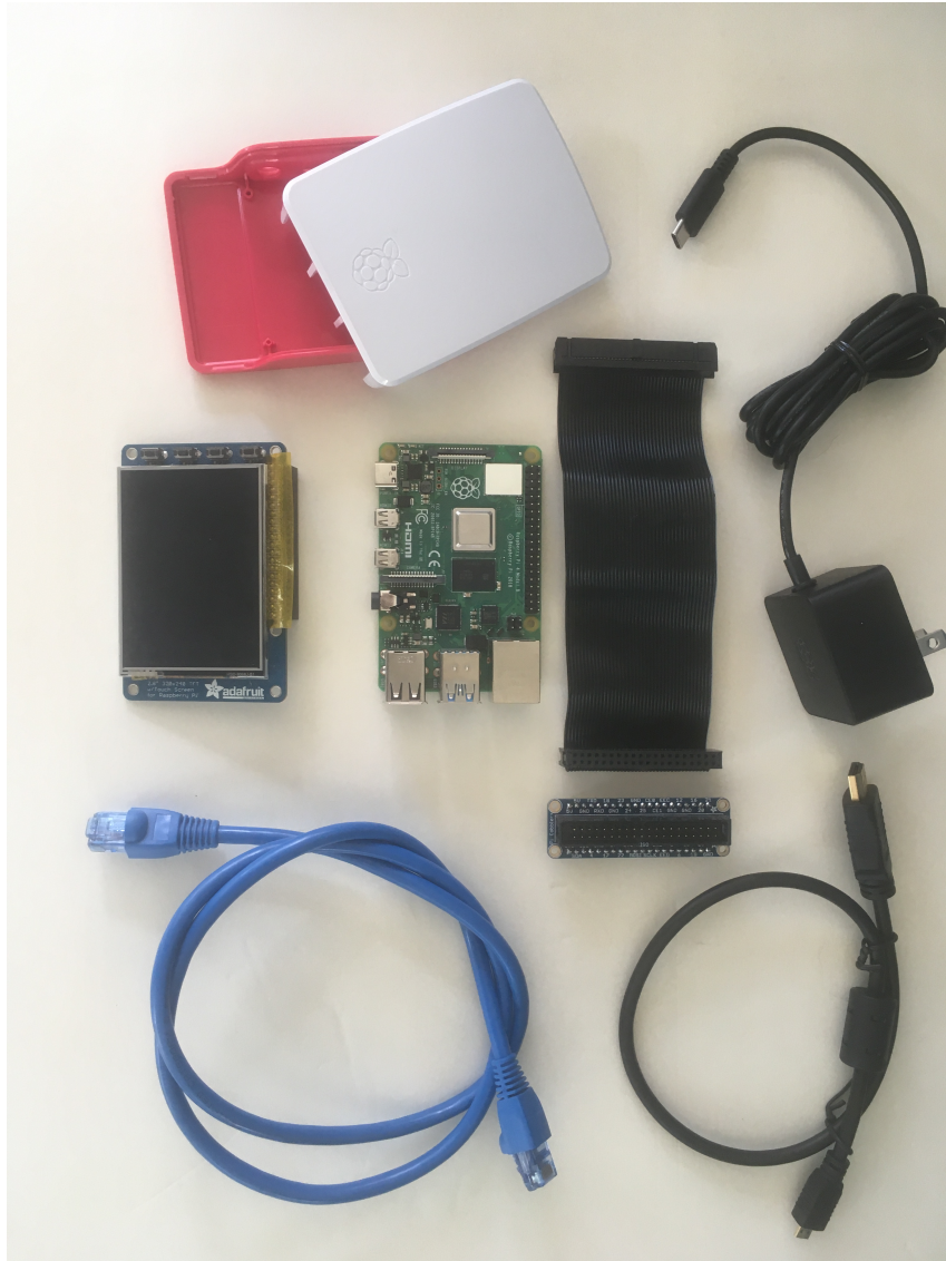
Elements of the ECE5725 Lab system: from top, left to right, RPi 4 case and cover, PiTFT display, RPi 4, Pi breakout cable and 40-pin cable header, 5V, 3.0 amp power supply, Ethernet cable, HDMI cable.
